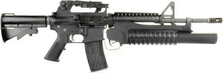
An M16 assault rifle equipped with an M203 40mm grenade launcher mounted on the front rail. The launcher has a distinctive ribbed barrel and a carrying handle. |
